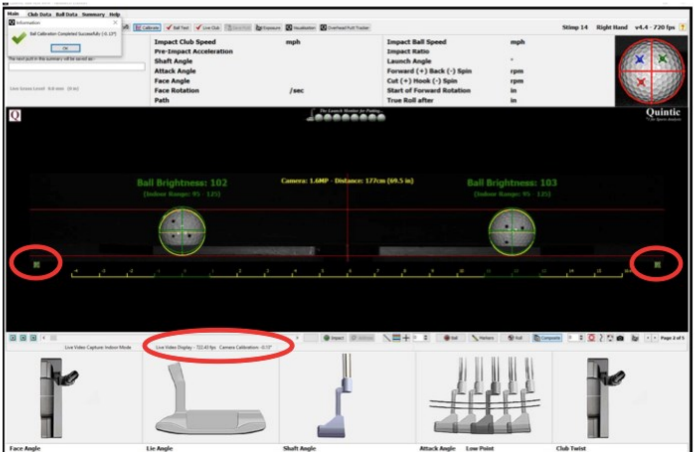
Figure 3: Calibration screen when all components of calibration were in the correct points.
